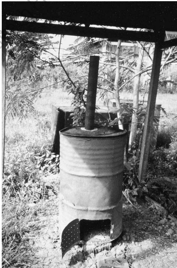
Fig. 8.6 Drum incinerator with chimney
